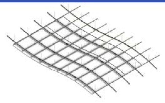
With the Hook-on System, it is much easier and safer to realize designs in special-sized panels.
